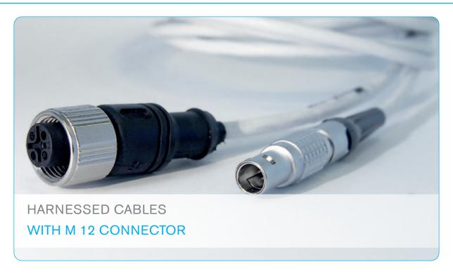
Harnessed sensor cable with a round plug connector and a M12 connector for the linking of the sensor (for example pressure sensor) with a module. The harnessed product can be designed according to the individual application. There are different plug and cable types available.
