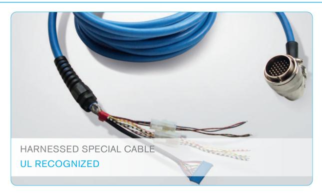
The shown product is equally used for the robot industry, particularly for paint robots. This type has got a 37-pole angle plug on the one side and an AMP Molex connector on the other side. According to the customer's requirements the cable harness can be adapted individually.
