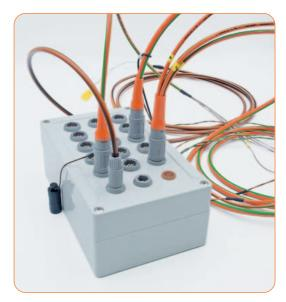
Connection box with fifteen 8-pole Redel sockets for thermal contacts and 2 NTC connections with 5-pole Redel socket. The box is used to connect HV sensors and to bundle all contacts on one potential. The voltage tap is made by a 4 mm safety socket.
