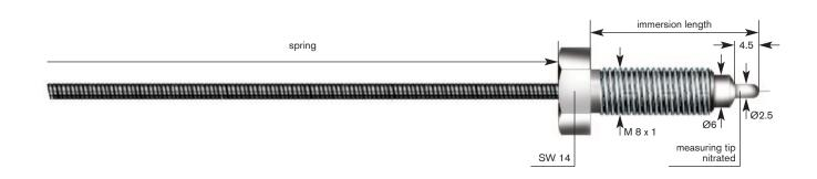
With the help of this special construction, the molten mass temperature in injection nozzles is measured. The surface treated measuring tip is also suitable for application in reinforced plastics. In case of adequate mounting only the nitrated measuring tip is in contact with the molten mass stream. Thus the temperature collection takes place directly in the mass without additional protecting sleeve.
